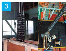
3 Chain is packaged folded on top of itself. Attach one end to a crane and lift out for easy removal.
