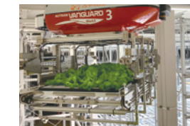
Autran Vanguard, an automatic handling system for plant factories (2021)
