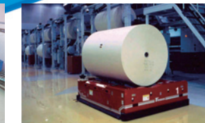
Automatic guided vehicle (AGV) paper feeding system, which has contributed to the automation of newspaper roll conveyors and the improvement of operations (1996)
