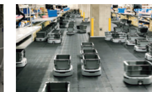
T-Carry System, a handling and sorting system using small AGVs (2020)
