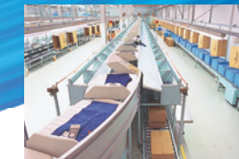
LiniSort, linear motor drive automated sorting equipment (1992)
