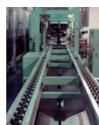
Plastic side roller chain developed for free flow conveyors (1981)
