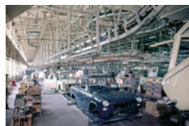
Noman Curve overhead conveyor delivered to an automobile plant (1961)
