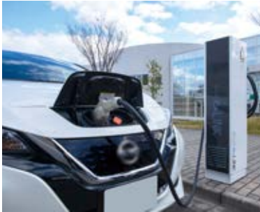
Connecting electric vehicles with emergency power supplies V2X bi-directional EV charging systems, eLINK
